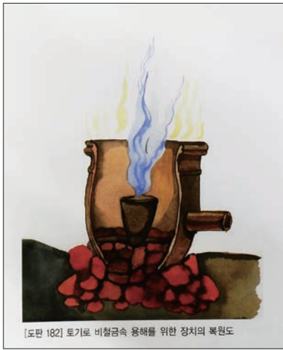
diagram 71. Is it the crucible method considered in Korea? This diagram is misused. The crucible loaded inside is not sealed.
